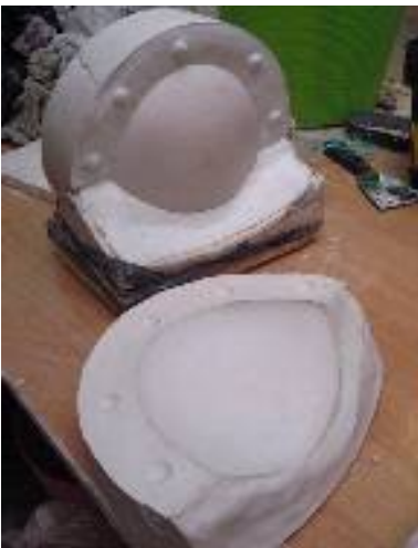
3-part slip mould for Yellow Bomb
