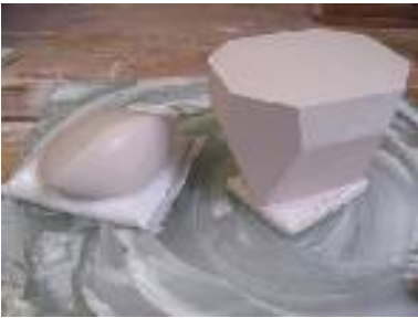
Plaster casts for slip-casting moulds
