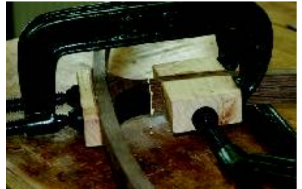
Gluing the joint
