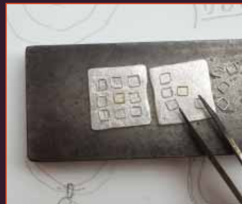
Shaping and placing the wires, Zsuzsi Morrison
